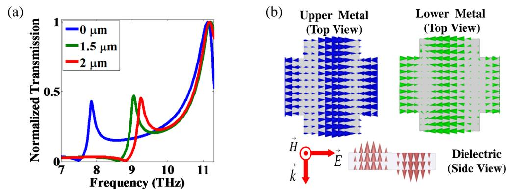
Figure 2: (a) Transmission characteristics of the FM showing shift in the negative peak with variation in the air gap thickness. (b) Instantaneous surface current and displacement current in top view of upper metallic layer, top view of lower metallic layer and side view of dielectric respectively at first peak.
