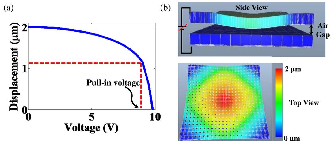
Figure 3: (a) Displacement versus Voltage graph showing pull-in voltage  $\cong 9$  V. (b) Side and top view of deformed membrane at pull-in voltage.
