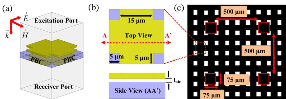
Figure 1: (a) Perspective view of unit cell of FM with boundary conditions used in electromagnetic simulation. (b) Top and Side view of a tunable FM unit cell along with geometrical dimensions. Thickness of air  $t_{air} = 0 - 2$   $\mu\text{m}$ . (c) Top view of repeating unit of top metallic layer with dimensions (not drawn to scale). Solid red boxes show the supporting pillars.
