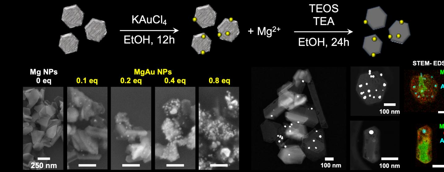
Galvanic replacement was monitored by Mg dissolution (ICP-MS) after decoration, and oxidation state (EELS) of single NPs.
