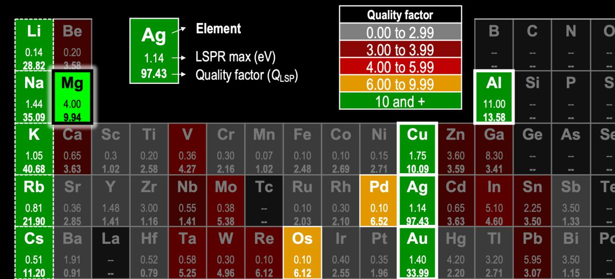
Noble metals have been the gold standards for plasmonic materials over the last millennia; however, the high cost of Ag and Au can be prohibitive in large-scale mainstream applications. Magnesium has been predicted to be an alternative offering:
